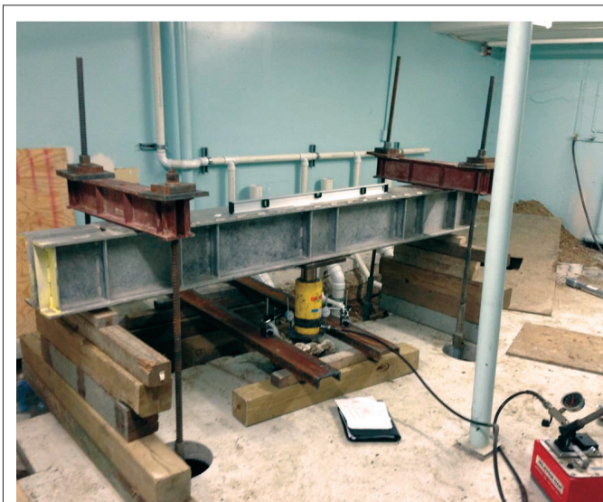
Indoor Compression Test Figure B-4
