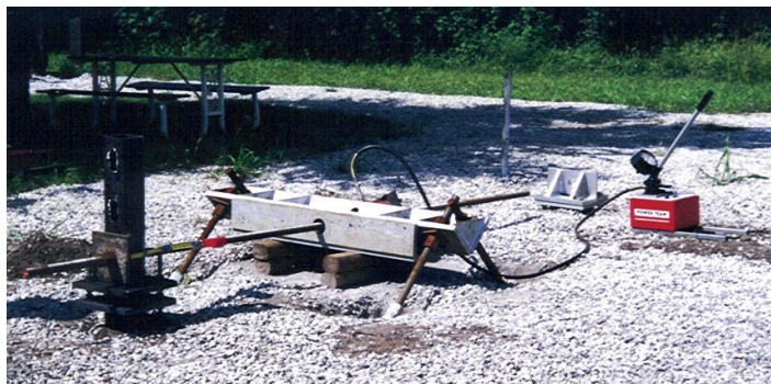
Lateral Load Test Apparatus Figure B-6
